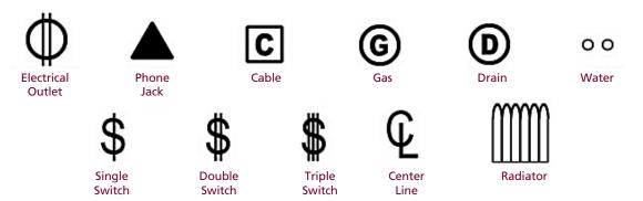
Please remember that service/utility locations are always measured to their centerline. Lastly, identify any obstructions that may create problems with the design (radiators, hood/exhaust vents, chimney chases and any heat registers).
